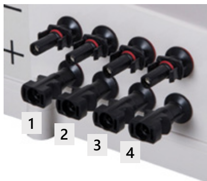
Figure 18. DC connection area, model 104, view from below
