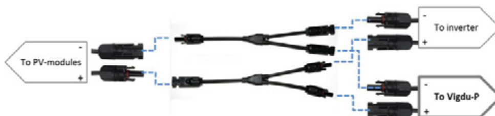
Figure 22. Connect Vigdu-P device with inverter and PV-modules
